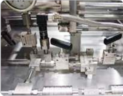
Back flushing system
